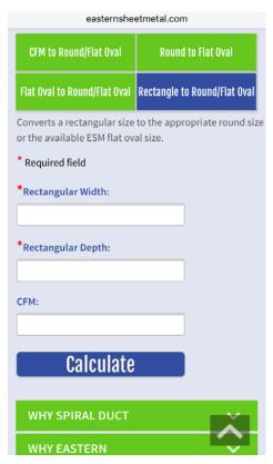
This option will calculate the equivalent round and flat oval dimensions for about five minor/major axis combinations, up to 36" minor axis, based on the rectangular size entered:
