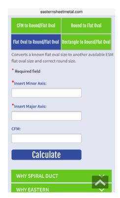
This option will calculate the equivalent round and flat oval dimensions for about five minor/major axis combinations, up to 36" minor axis, based on the flat oval size entered:
