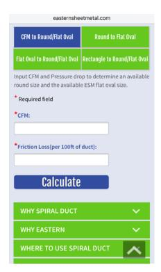
This option will calculate a round size and several equivalent flat oval dimensions in inches for about six minor/major axis combinations. For example if you want to use a 0.20 per 100 ft friction loss and 5000 cfm the program will calculate:
